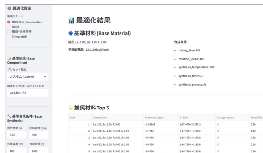
Fig. C.7. Data-driven inference and recommendation of next candidate compositions and synthesis conditions.
