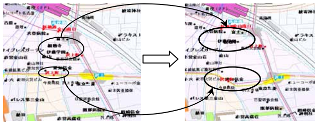
Fig 2 The Context Aware Map Synthesizer introduces new conflicts between the labels when slight scale changes are made
